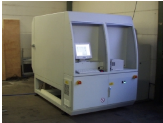
Figure 9: Shearography Measurement System Front with Operator's Desk
